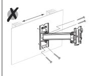
Ensure that the mount is fixed to a solid object and not into plasterboard on its own.
