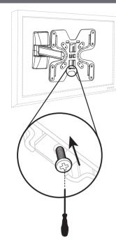
Using a screwdriver tighten the securing bolts onto the mount.
