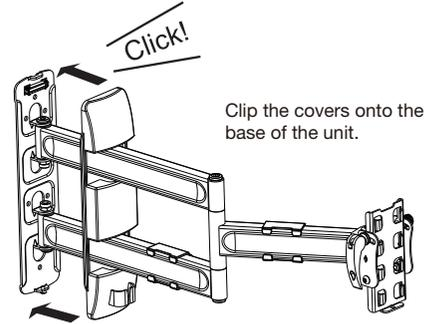
Clip the covers onto the base of the unit.
