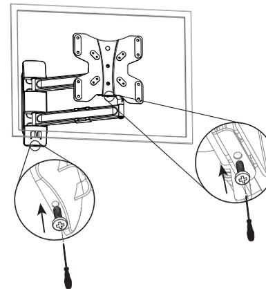
Using a screwdriver tighten the securing bolts onto the mount and the bottom of the cover.
