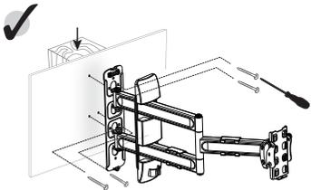
Using the provided self tapping screws (B) type. Holding the TV mount starting in the one corner, screw the provided screws (B) into a wooden joist fixing the opposite corners, until the mount is secure onto the wall. Ensure all are tight and secure.
