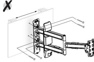
Ensure that the mount is fixed to a solid object and not into plasterboard on its own.
