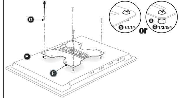
Provided select the appropriate ones to hold the hooks (G) onto the TV. Ensuring that the mounts are facing the the top end of your TV screw the mount onto the TV ensuring not to over-tighten.
