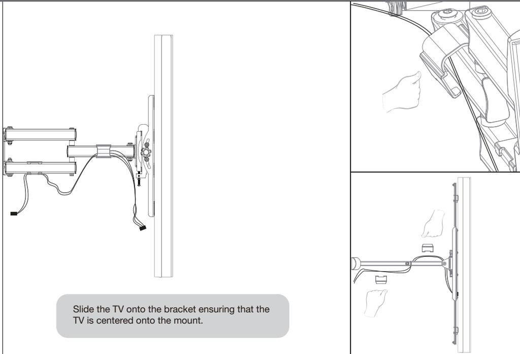
Slide the TV onto the bracket ensuring that the TV is centered onto the mount.
