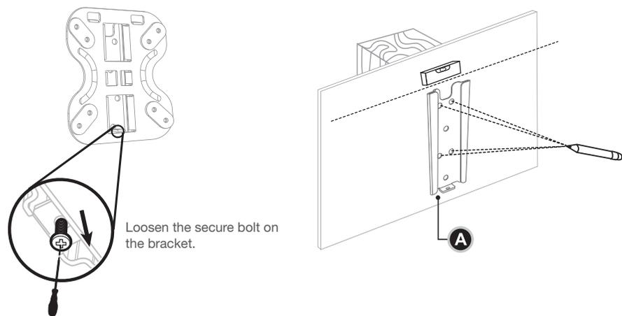
Loosen the secure bolt on the bracket.
