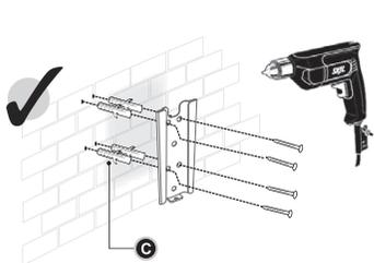
When selecting the position of the TV mount, ensuring that the mount will be mounted on to a flat surface and is level. Mark the wall where the fixing locations are. Drill the holes using a 10mm masonry bit. Using a hammer knock the the wall plugs (C) provided into the wall. Holding the TV mount start in the one corner screw the provided screws (B) into the wall fixing the opposite corners until the mount is secure onto the wall. Ensure all are tight and secure.
