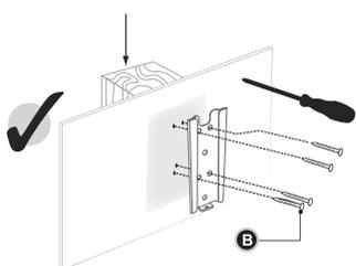
Using the provided self tapping screws (B) type. Holding the TV mount starting in the one corner, screw the provided screws (B) into a wooden joist fixing the opposite corners, until the mount is secure onto the wall. Ensure all are tight and secure.
