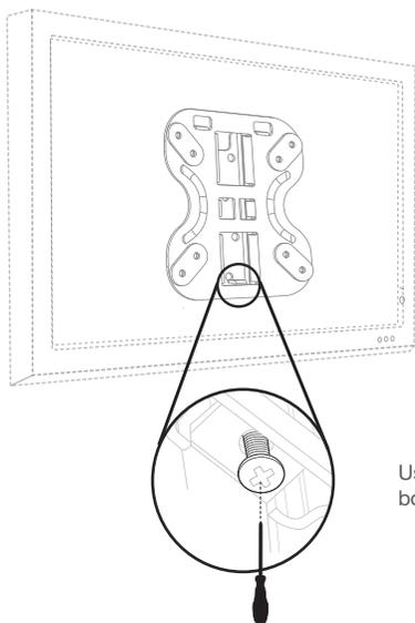
Using a screwdriver tighten the securing bolts onto the mount.
