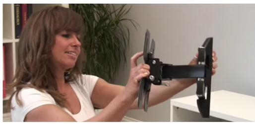
Separate the parts of the mount which attach to the TV from the parts which mount to the wall (there may be a screw holding them together).
