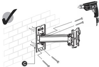
When selecting the position of the TV mount, ensuring that the mount will be mounted on to a flat surface and is level. Mark the wall where the fixing locations are. Drill the holes using a 10mm masonry bit. Using a hammer knock the the wall plugs (C) provided into the wall. Holding the TV mount start in the one corner screw the provided screws (B) into the wall fixing the opposite corners until the mount is secure onto the wall. Ensure all are tight and secure.
