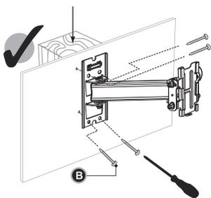
Using the provided self tapping screws (B) type. Holding the TV mount starting in the one corner, screw the provided screws (B) into a wooden joist fixing the opposite corners, until the mount is secure onto the wall. Ensure all are tight and secure.
