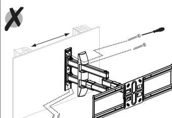
When selecting the position of the TV mount ensure that it is fixed onto a wooden joist or onto a solid wall. Mark the wall where the fixing locations are ensuring that the mount will be mounted on to a flat surface and is level.
