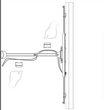
Slide the TV onto the bracket ensuring that the TV is centered onto the mount.
