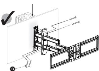
Using the provided self tapping screws (B type). Holding the TV mount starting in the one corner, screw the provided screws (B) into a wooden joist fixing the opposite corners, until the mount is secure onto the wall. Ensure all are tight and secure.
